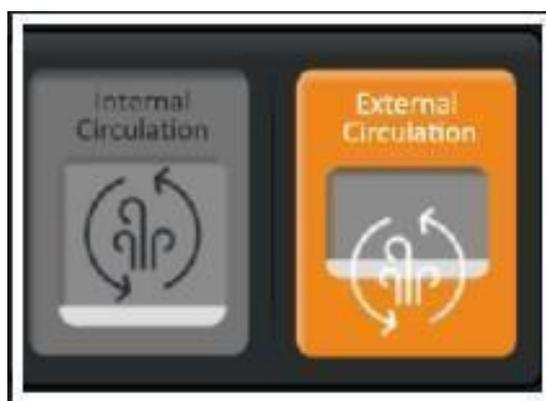
When the ICU is turned on, the default mode is **External Circulation (also known as ‘A Mode’)**, and the icon that indicates this is highlighted in orange when active. Under this setting, the oxygen concentration in the air within the inside and outside of the ICU chamber is the same due to the ventilation that is taking place. To switch from ‘External Circulation’ to ‘Internal Circulation’, you may click the icon labeled “Internal Circulation” to turn on the Internal Circulation Mode.
